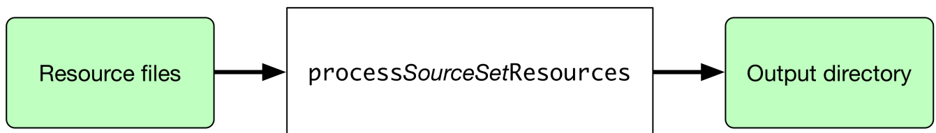
Figure 26. Processing non-source files for a source set
