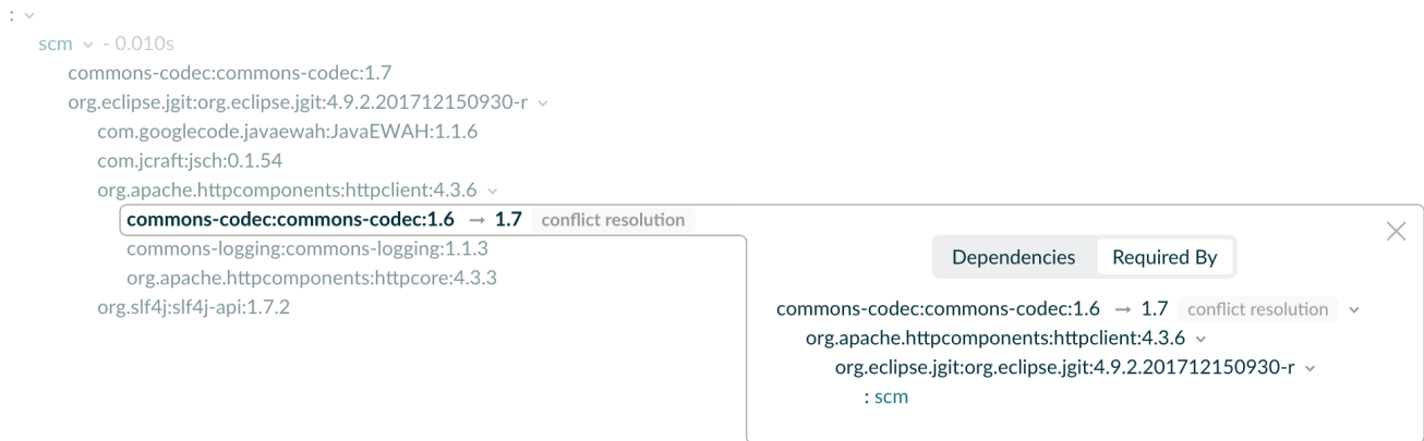
Figure 20. Dependency insight capabilities in a build scan
